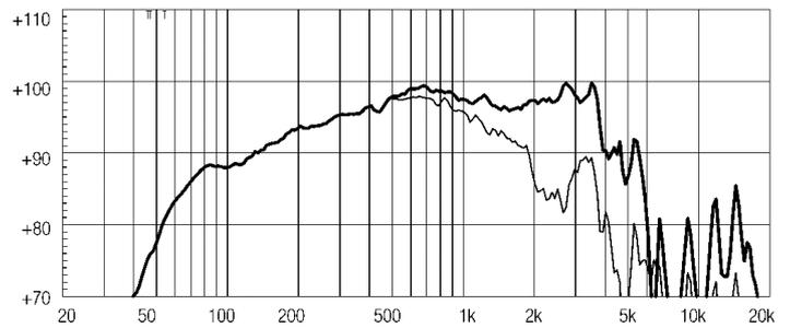
**FREQUENCY RESPONSE CURVE OF 10MB600 MADE ON 30 LIT. ENCLOSURE TUNED AT 55HZ IN FREE FIELD (4PI) ENVIRONMENT. ENCLOSURE CLOSES THE REAR OF THE DRIVER. THE THIN LINE REPRESENTS 45 DEG. OFF AXIS FREQUENCY RESPONSE FREE AIR IMPEDANCE MAGNITUDE CURVE**
